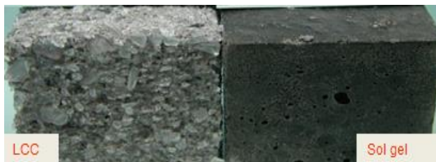
Fig. 13: Resistance to acids of LCC/sol-gel bonding
