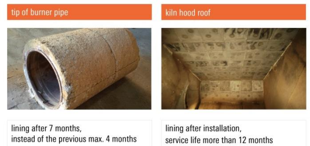
Fig. 8: Cement-free andalusite geopolymer bonded concrete in highly loaded areas of cement plants
