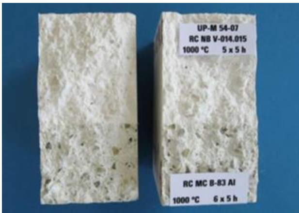
Fig. 9: Sample preparation for the evaluation of the bonding strengths in the contact zone: MCC (bauxite) sol-gel (WFA) concrete after pre-firing at 1000 °C/5 h. Separation by MOR of 21 MPa through concrete structure, no separation in the contact zone.
